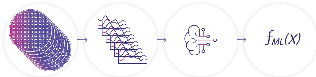
Figure 2. The MapPro training flow. We start with several dozen densely measured wafers. This data is used for training the ML algorithm where for the labeling we use the qualified OCD solution. After the training stage we obtain an ML model that can be run on the measuring tool and publish the results to the host.
