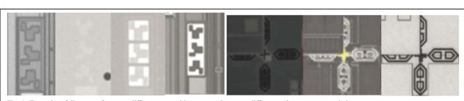
Fig. 4. Examples of die corner feature at different steps with pattern and contrast differences due to process variation.
