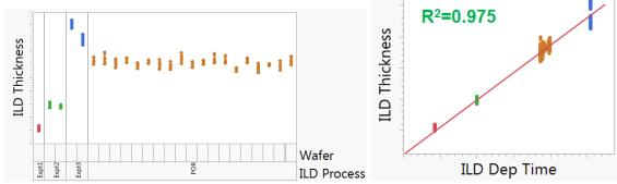
Figure 9: Measurement of ILD thickness by ILD process grouping and correlation of ILD thickness to ILD dep time
