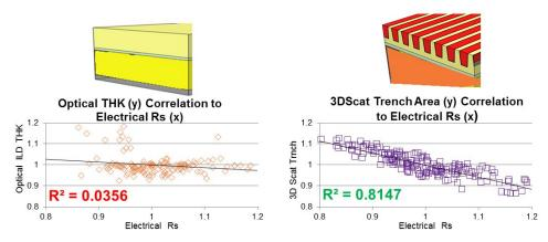
Figure 1: Comparison of correlation of 1D optical measurement and 3D scatterometry measurement to electrical resistance parameter [1]
