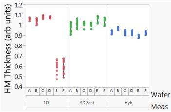
Figure 3: Comparison of 10x precision measurements of hard mask thickness for six 14nm wafers by 1D optical, 3D scatterometry and hybrid scatterometry measurement techniques
