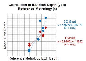
Figure 8: Correlation of hybrid scatterometry and 3D scatterometry ILD etch depth to reference metrology.
