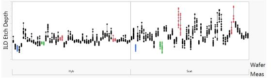
Figure 7: Comparison of hybrid scatterometry and 3D scatterometry ILD etch BCD measurements for 7nm wafers.
