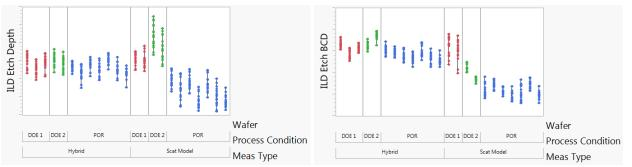
Figure 6: Comparison of hybrid scatterometry and 3D scatterometry ILD etch depth and BCD measurements for 14nm wafers.
