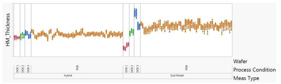
Figure 5: Comparison of hybrid scatterometry and 3D scatterometry hard mask thickness for 14nm wafers including incoming process DoE conditions.
