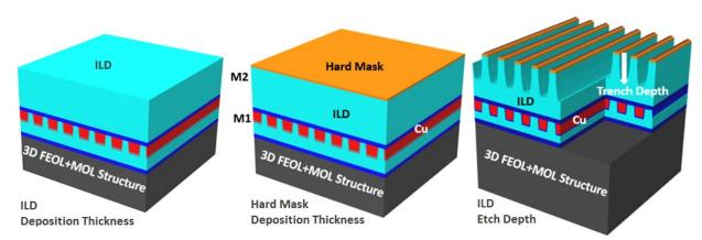
Figure 2: Schematic of measurement structure used for interlayer dielectric (ILD) thickness, hard mask thickness and interlayer dielectric trench depth measurements.
