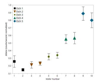
Fig. 5. Ge  $L\alpha$  count difference from pre and post indentation measurements as a function of wafer number. The individual data points are wafer averages and the error bars indicate the within wafer variation. An increasing  $\Delta Ge L\alpha$  corresponds to an increasing lateral SiGe etch.
