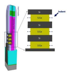
Fig. 1. Schematic drawing of a stacked nanosheet FET unit cell after SiGe indentation. The highlighted 2D section details the alternating Si and SiGe sheets with the lateral etch of the sacrifical SiGe.
