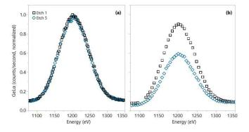
Fig. 4. Ge  $L\alpha$  counts as measured by LE -XRF, both (a) before and (b) after the indentation, for two of the different DOE conditions, Etch1 and Etch5.
