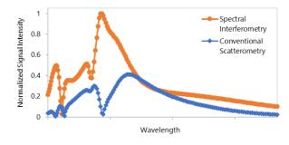
Fig. 2. Normalized signal intensity variation as a function of wavelength for conventional scatterometry and Spectral Interferometry channels when the SiGe indent parameter is varied by 1 nm.
