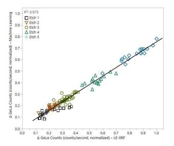
Fig. 7. Comparison of  $\Delta Ge\ L\alpha$  between machine learning based scatteromerty (post indent metrology only) and LE-XRF metrology (pre and post indent metrology).
