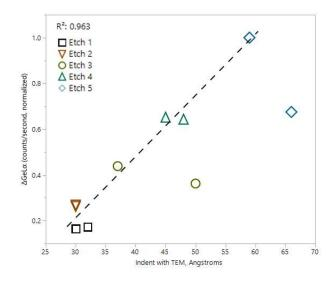
Fig. 6. Comparison of LE-XRF ( $\Delta Ge \ L\alpha$ ) and TEM results for the indent. The dashed linear fit line is calculated without the two outliers (TEM = 50 Å and 66 Å).
