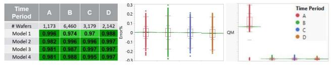
Figure 11. R<sup>2</sup> matrix, Error % and QM trend for thin film thickness measurement by improved throughput ML model.
