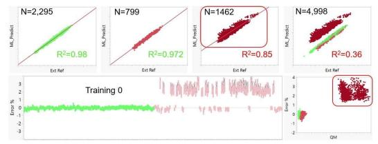
Figure 8. R<sup>2</sup>, Error % and QM for thin film thickness prediction from Model 1 applied on training and blind test samples.
