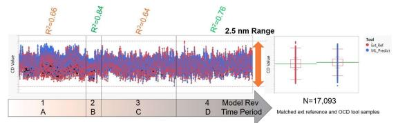
Figure 3. ML Predicted CD (labelled as ML\_Predict) and external CD reference (labelled as Ext\_Ref) show close baselines with a ~2.5 nm range. For 17,093 sampling dies, the averaged ML predicted CD has 0.6% higher mean, and 9.9% lower overall standard deviation than the external CD reference.
