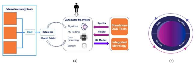
Figure 1. (a) Schematic of the ML eco-system to create, retrain and monitor ML metrology solutions, with significantly reduced human operations; (b) Data process flow in this ML eco-system.
