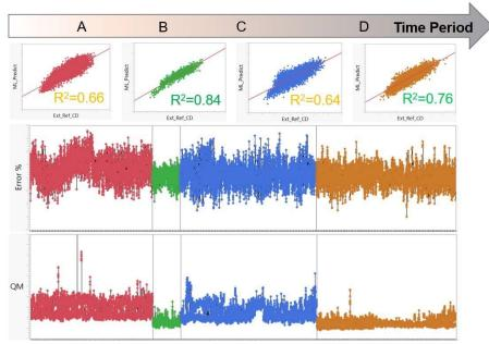
Figure 4. R<sup>2</sup>, Error % and QM trend for fin CD prediction during blind test.
