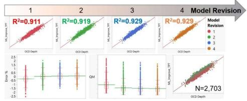
Figure 12. R<sup>2</sup>, Error % and QM trend for thin film thickness measurement by throughput optimization ML model.
