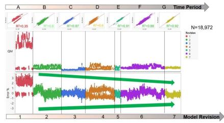
Figure 7. R<sup>2</sup>, Error % and QM trend for thin film thickness prediction during blind test
