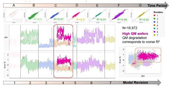
Figure 9. R<sup>2</sup>, Error % and QM for thin film thickness prediction highlighting high QM wafers in time period D by Model 4.
