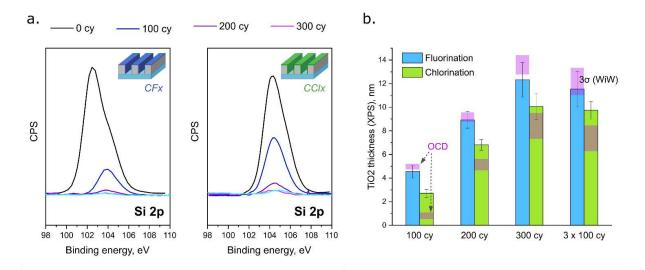
Figure 6. XPS analysis of the ASD  $TiO_2$  process on the growth area (SiN<sub>x</sub>) in the 90 nm pitch a-C:H line pattern: (a) evolution of Si 2p peak induced by deposition of ALD  $TiO_2$ ; (b)  $TiO_2$  thickness estimated via attenuation of Si 2p peak intensity and corresponding OCD  $TiO_2$  thickness.
