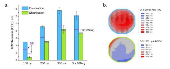
Figure 4. OCD analysis of the ASD  $TiO_2$  process on the growth area (SiN<sub>x</sub>) at the 90 nm pitch a-C:H line pattern: (a) OCD  $TiO_2$  thickness in comparison with the results of spectroscopic ellipsometry (SE) measurements performed at SiN<sub>x</sub> pattern-free areas of the same wafer; (b) OCD  $TiO_2$  thickness wafer map.
