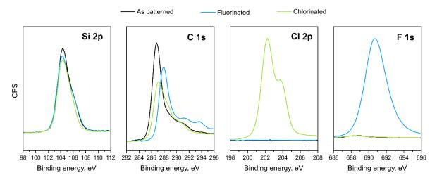
Figure 5. High-resolution XPS scans for representative element peaks recorded on 90 nm pitch a-C:H line pattern before and after the plasma halogenation.
