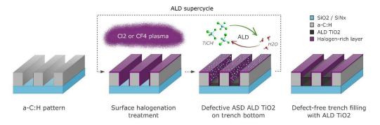
Figure 1. The proposed approach for area-selective deposition of ALD TiO<sub>2</sub> featuring plasma halogenated amorphous carbon as a non-growth surface and an ALD supercycle scheme based on intermediate halogenation plasma treatment.
