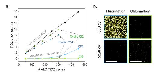
Figure 2. Selectivity and defectivity of the proposed ASD ALD TiO<sub>2</sub> process tested on blanket films: (a) thickness of ALD TiO<sub>2</sub> measured on SiO<sub>2</sub> and on halogenated amorphous carbon surfaces with RBS; (b) defect map obtained from AFM topography images by threshold marking ( $5\sigma$ ), the scalebar on the images is 500 nm.
