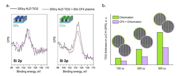
Figure 8. Adverse effect of hard-mask residues on selectivity of ALD  $TiO_2$  process featuring chlorinated a-C:H line pattern: (a) Si 2p XPS signals recorded after deposition of 300 cycles ALD  $TiO_2$  and after additional exposure to CF<sub>4</sub> plasma; (b) the effect of CF<sub>4</sub> plasma pre-treatment on the  $TiO_2$  defects formed over the non-growth area (chlorinated a-C:H) assessed by XPS and top-down SEM.
